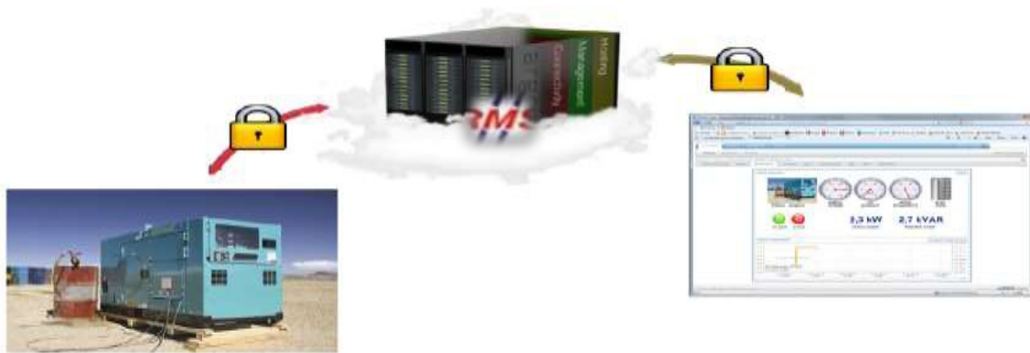
A secure and reliable remote management solution requires encryption both between the power generator in the field and the data center as well as between the data center and the web interface.
